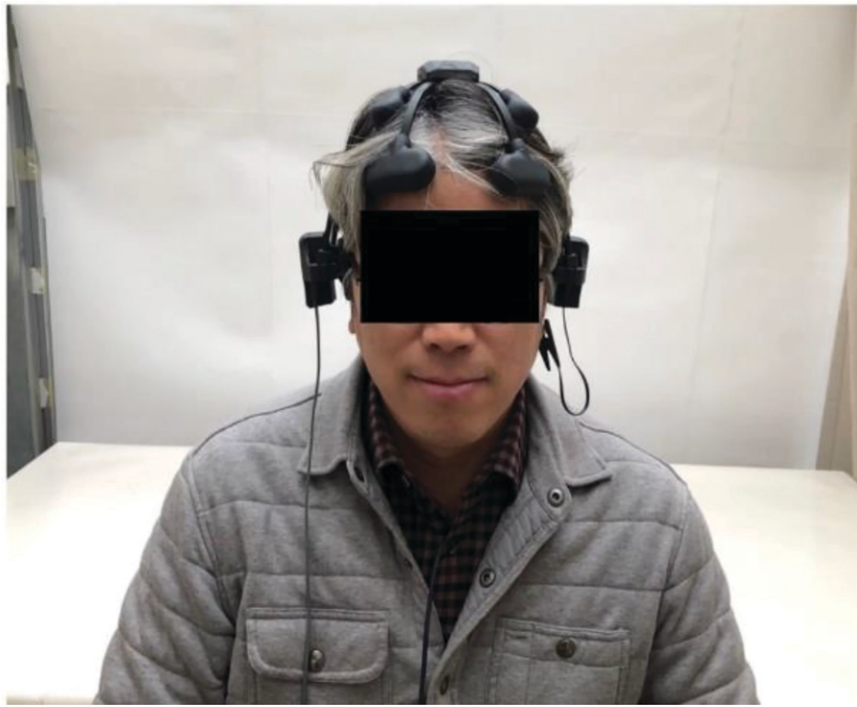
Fig. 4. Dry EEG wireless electroencephalography device (Quick-20; Cognionics, San Diego, CA).
